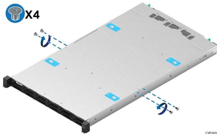
Figure 74. System Top Cover Panel Shipping Screws
