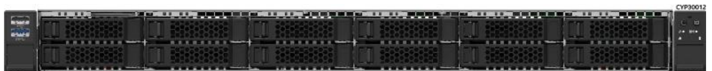
Figure 64. 12 x 2.5" Front Drive Bay Configuration
