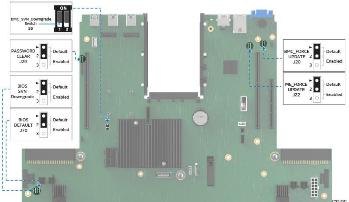
Figure 73. Reset and Recovery Jumper Block Locations
