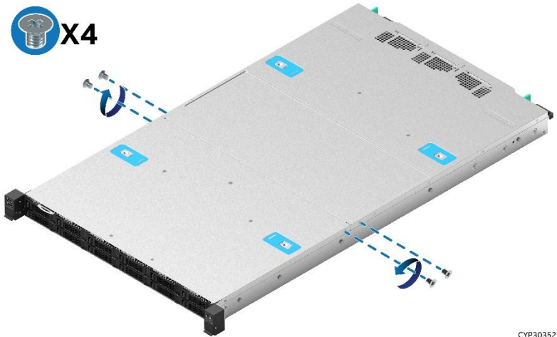
Figure 2. System Top Cover Panel Shipping Screws
