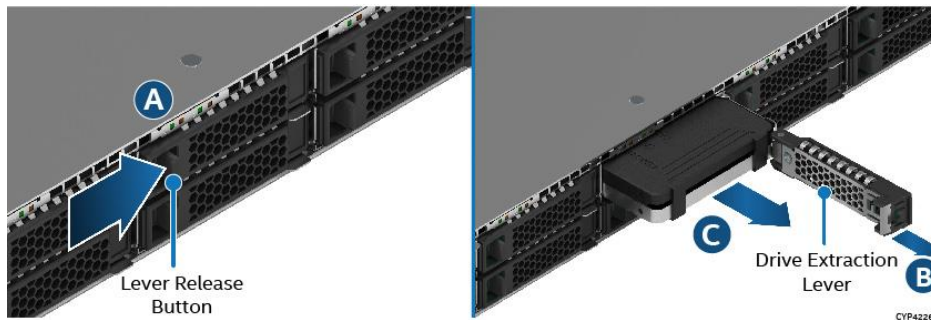
Figure 97. 2.5" 7 mm Drive Removal
