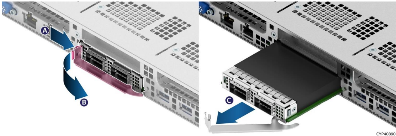
Figure 45. OCP* Adapter with Ejector Latch Removal
